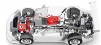
1. Power electronics 2. Power axle with two electric motors 3. High-voltage cable 4. Electric synchro-race battery 5. Power electronics
